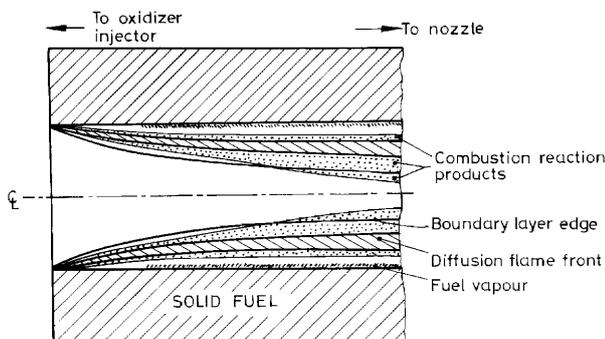
**Fig. 6 Combustion processes in hybrid rocket motor.<sup>13</sup>**
