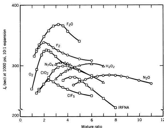
**Fig. 2** Theoretical vacuum specific impulse of selected liquid oxidizers and hydroxyl-terminated-polybutadiene solid fuel (adopted from Ref. 1)
