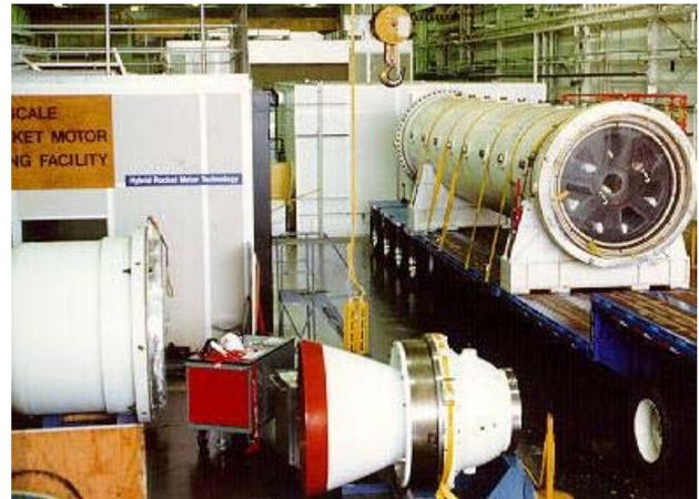
**Fig. 8 Hybrid motor assembly at NASA- Marshall — note the wagon wheel grain configuration for the fuel grain (adopted from www.nasa.gov).**
