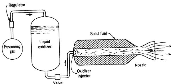
**Fig. 1** Simplified schematic diagram of typical hybrid rocket engine (adopted from Ref. 1)
